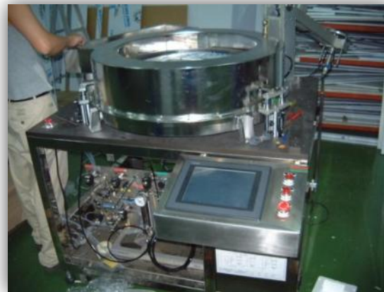
320x400mm玻璃基板光阻塗佈用 For 320x400mm glass PR coating
