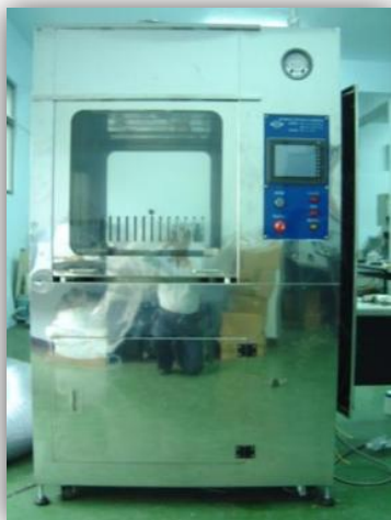
4吋基板光阻塗佈用 For 4in wafer PR coating
