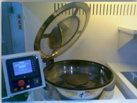
285x305mm玻璃基板光阻塗佈用 For 285x305mm glass PR coating
